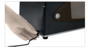
Plug the end of the Pneumatic Connection into the air connector on the back of the module; then connect the nipple for the Pneumatic Connection to the air supply. Set the air pressure of the air supply to 5-10 bars.
